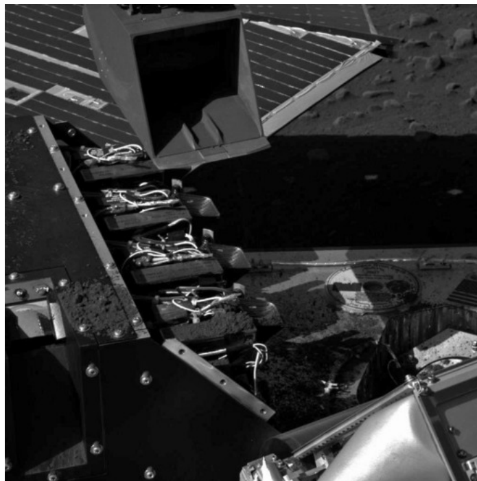
This image taken by the Surface Stereo Imager on NASA's Phoenix Mars Lander shows the lander's Robotic Arm scoop positioned over the Wet Chemistry Lab Cell 1 delivery funnel on Sol 41, the 42nd Martian day after landing, or July 6, 2008, after a soil sample was delivered to the instrument.
