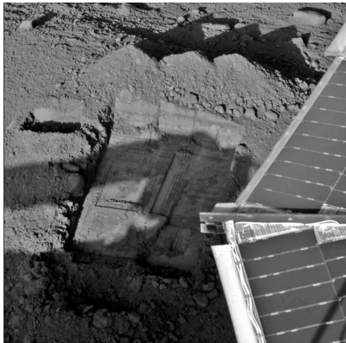
This image was acquired by NASA's Phoenix Mars Lander's Surface Stereo Imager on the 44th Martian day of the mission, or Sol 43 (July 7, 2008), after the May 25, 2008, landing, showing the current sample scraping area in the trench informally called "Snow White." Image credit: NASA/JPL-Caltech/University of Arizona/Texas A&M University
